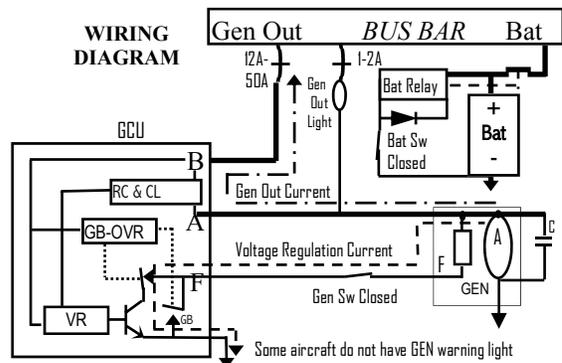
**Caution:** Check the condition of the battery. A depleted /discharged battery will draw excessive current and could trigger the Current Limiter function to turn off the GCU's voltage regulator.
